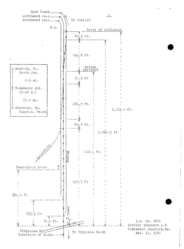
the south switch of the cross-over connecting the two main tracks. The cross-over switches to the spur track are hand operated, and all other switches mentioned are interlocked and operated from Tidewater Junction tower.
